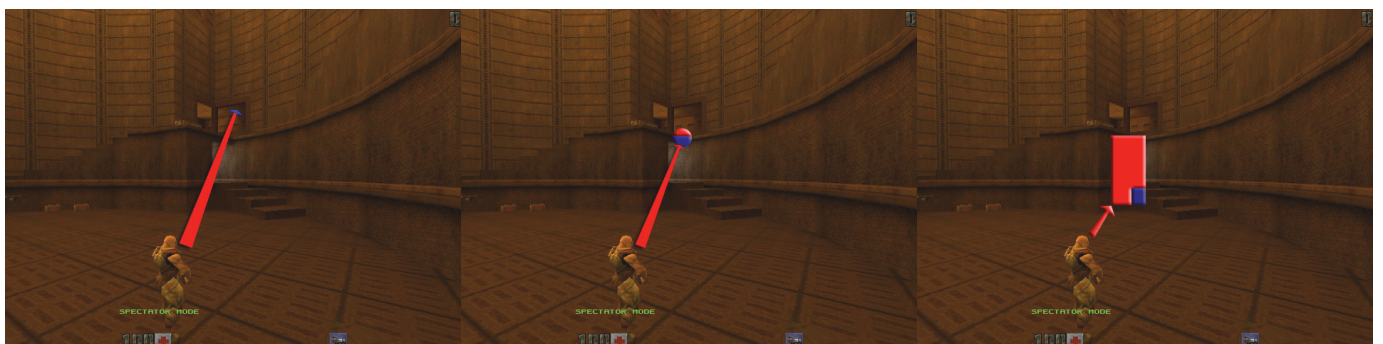
Figure 4 - BSP traces with line, sphere and box. Collision occurs at different points.
